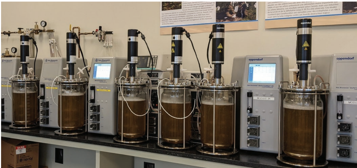
Native strains of endophytic fungi growing in bioreactors for seedling inoculation to help trees tolerate insect pests.
